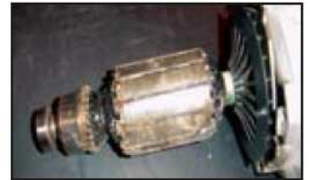
Armature burnt out (overloaded)
