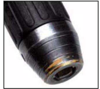
Wear caused by operating the drill with the chuck running against masonry or other hard surfaces
