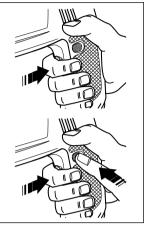
To switch your drill on, depress the on/off switch. Your drill stops when the on/off switch is released. If continuous operation is required, depress the lock-on button while the on/off switch is depressed. To stop your drill when operation is continuous, depress the on/off switch
