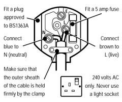
Before replacing the top cover of the plug ensure that the cable restraint is holding the outer sheath of the cable firmly and that the two leads are correctly
