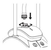
6. Place the steam head onto the steam head support on the clothes hanger.
