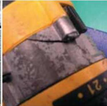
Cracks on dropped unit
