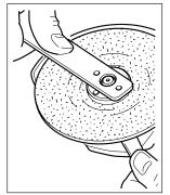
Remove the guard. Place the flange on the spindle. Place the backing pad on the spindle and inner flange, ensuring it is correctly located. Mount the fibre backed abrasive disc on the backing pad.
