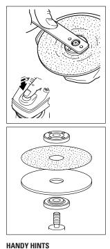
Fit the threaded outer flange and tighten as explained in 'Fitting the discs'.
