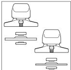
Fit the threaded outer flange (b), making sure it is facing in the correct direction for the type of disc fitted. For grinding discs, the flange (b) is fitted with the raised portion facing
