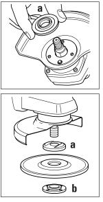
two flats. Place the abrasive disc on the spindle and
