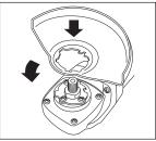
Place the angle grinder on a table, spindle up. Align the lug with the slot in the bracket. Press the guard down and turn it in the direction of the arrow.
