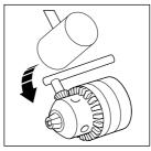
To remove the chuck, open the jaws of the chuck with the chuck key. Hold the chuck firmly in one hand, and with a screwdriver turn the screw set in the chuck clockwise with the other hand until it comes out.
