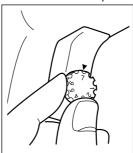
Set the speed of your drill. Set the variable speed control to the desired position. As a general rule, for large size drill bits use low speeds and for smaller drill bits use high speeds.
