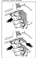
To switch your drill on, depress the on/off switch or the variable speed switch. Your drill stops when the on/off switch or the variable speed switch is released. If continuous operation is required, depress the lock-on button while the on/off switch or variable speed switch is depressed. To stop
