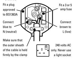
Before replacing the top cover of the plug ensure that the cable restraint is holding the outer sheath of the cable firmly and that the two leads are correctly fixed at the terminal screws. If the fuse cover is missing or damaged do not use the plug.
