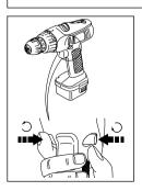
The forward/reverse and lock-off switch controls the direction of rotation of the chuck. In the centre position, it prevents starting of your drill when changing accessories or during storage.
